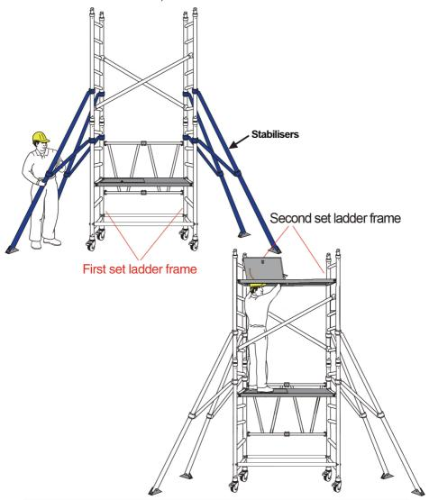
7. Repeat Step 2. Add the platform with hatch to the 2<sup>nd</sup> rung of the second set of the 6 rung ladder frame. Lock the platform.
