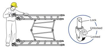
2. Stand the Base unit upright with the support of two persons. Once the frame has been put into the open position, you are then able to locate the platform with hatch onto the 3<sup>rd</sup> rung of the 6-rung ladder (count from the bottom to the top). Lock it in place and inspect the stability.
