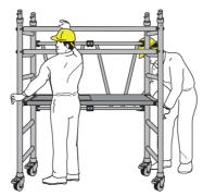
3. Locate the two guard rails onto the 5<sup>th</sup> and 6<sup>th</sup> rungs to provide additional safety and support.
