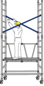
5. Locate the diagonal braces. Clip the diagonal braces onto the lowest rung of the Tower frame and angle across to the opposite frame. The Tower set up is now self-supported and steady.
